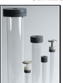
Griffco Borosilicate Glass Calibration Cylinders are designed to enhance the performance of chemical feed systems by providing a verification of the flow rate of the chemical feed pump. Constructed of borosilicate glass and a choice of 8 end cap materials, (PVC, CPVC, PP, PTFE, PVDF, 316SS, Alloy 20, and Hastelloy C) these cylinders are suitable for use with most chemicals. Available in 12 sizes: from 30mL to 20 L.
